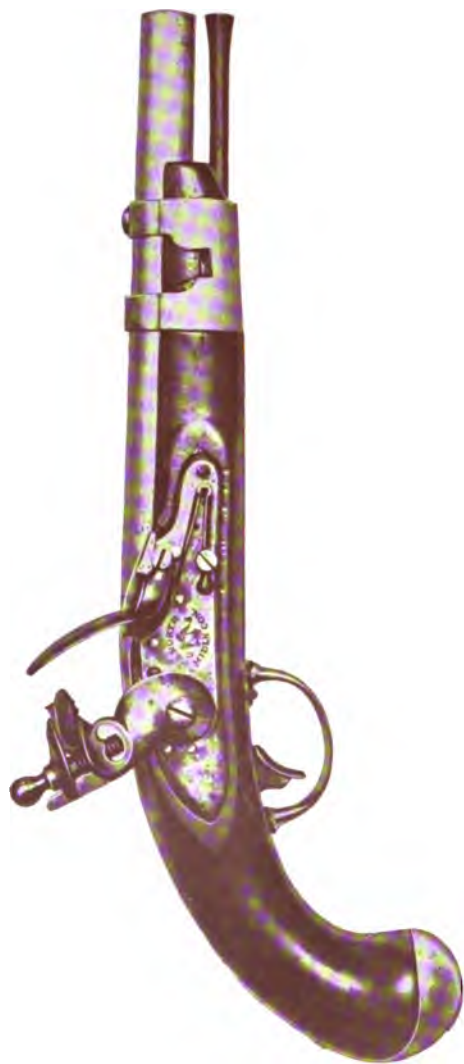
Horse pistol; model of 1813, as modified in 1816. Length 15½ inches. Length of barrel 9 inches. Caliber, 54. Sight on band. Iron mountings.
